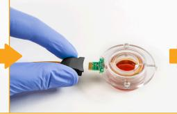
The inovitro live cable is connected to the insert.
