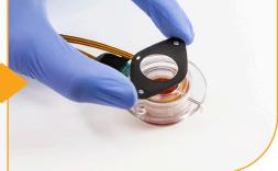
The cover heating element with temperature control is secured over the inovitro live insert.
