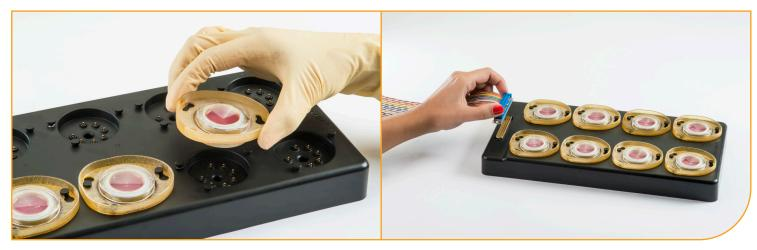
The ceramic dishes (8) are plugged into the **base plate**, which connects to the **TTFields generator** through a **flat cable**.
