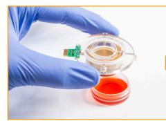
The inovitro live insert is inserted into the high-wall glass-bottom petri dish.
